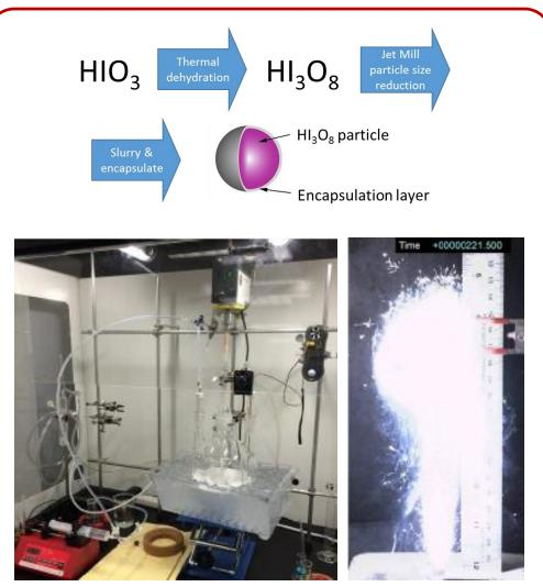
Microparticle synthesis & combustion in thermite; combustion test courtesy of Prof. T. Weihs, Johns Hopkins University
