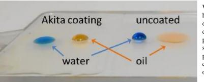
Water (dyed blue) and hexadecane (oil; dyed orange) droplets on an Akita coating (left) and bare polycarbonate (right), showing the unusual property of hydrophilicity combined with oleophobicity.
