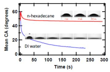
Contact angle of hexadecane (red) and water (blue) as a function of time on an Akita antifog coating. Insets: droplet photos
