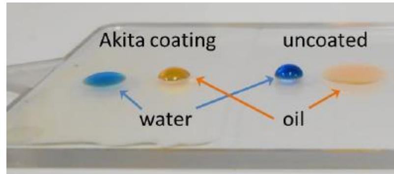
Water (dyed blue) and hexadecane (oil; dyed orange) droplets on an Akita coating (left) and bare polycarbonate (right), showing the unusual property of hydrophilicity combined with oleophobicity.
