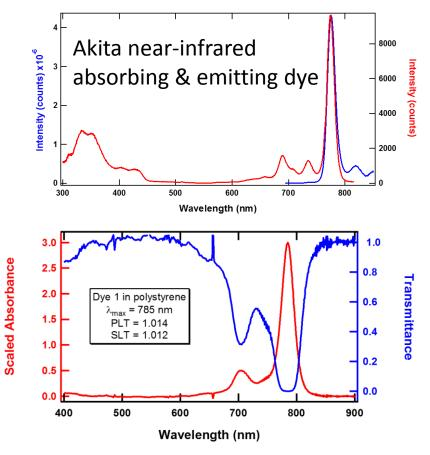
Laser-line absorber with high visible transmittance
