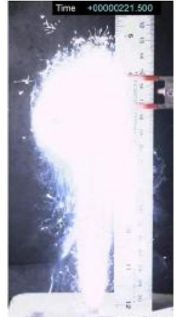
Microparticle synthesis & combustion in thermite; combustion test courtesy of Prof. T. Weihs, Johns Hopkins University
