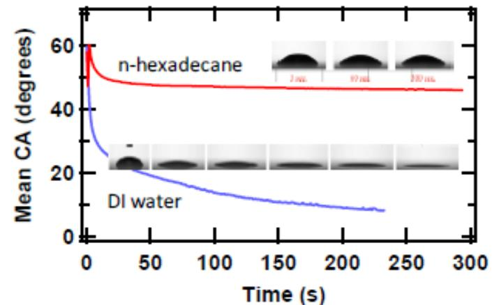
Contact angle of hexadecane (red) and water (blue) as a function of time on an Akita antifog coating. Insets: droplet photos
