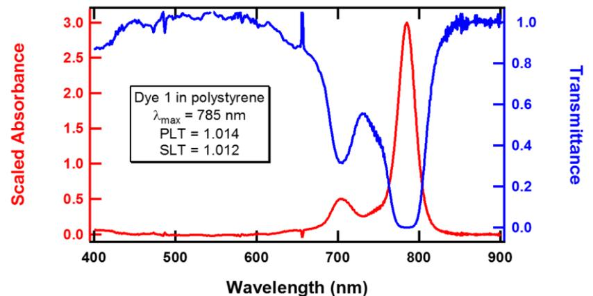
Laser-line absorber with high visible transmittance
