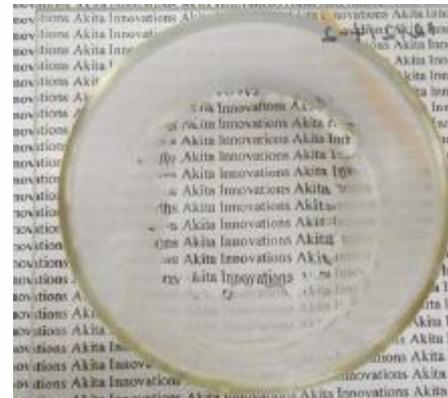
'Steam test' at 40°C showing anti-fog effect of Akita coating (center of slide).
